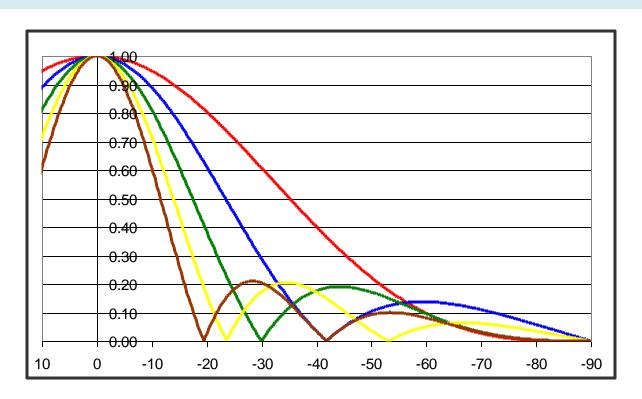
Typically a 4- or 5-bay antenna on a 200 foot structure would be used where population is just a few hundred feet away. But what if your design placed higher RF levels over just one or two houses near the tower? ... The second way we can solve the problem is with the relative pacing of the antenna bays.
